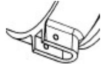
Position the Nozzle Tip so the control cable loops are hanging down. Attach one of the swivel snap hooks from the long nozzle control cable assembly to one of the cable loops on the nozzle. Attach the other swivel snap hook to the remaining loop on the nozzle.
